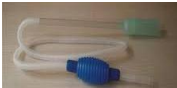
Figure 3.15: Siphon used for the experiments (author, 2012)
