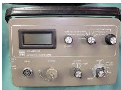
Figure 3.12: YSI Model 58 dissolved oxygen lab meter (author, 2012)
