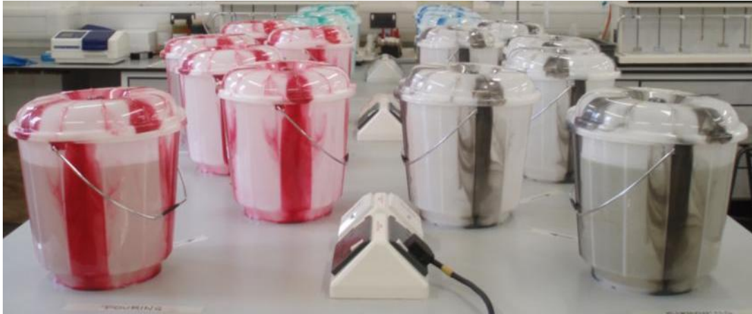
Figure 3.13: Experimental setup: Pouring systems in red (right front side) – Siphoning systems in black (left front side) – Control pouring systems in green (right back side) – Control siphoning systems in blue (left back side) (author, 2012)
