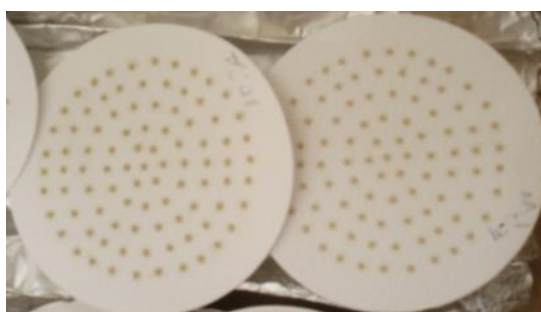
Figure 3.11: Suspended solids Glass microfiber paper filters in use (author, 2012)
